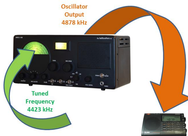
Figure 21. A Tecsun PL-660 Used to Tune a Hallicrafters S-40B to Specified Frequency
