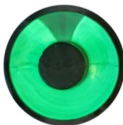
Figure 3. Magic Eye Tuning Tube
